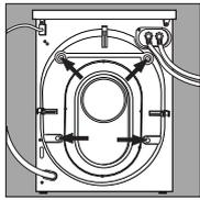
Before using the washer-dryer, **remove the screws**, remove the spacers together with the rubber tubes attached to them (keeping all the parts) and use the plastic plugs provided to fill in the holes.
